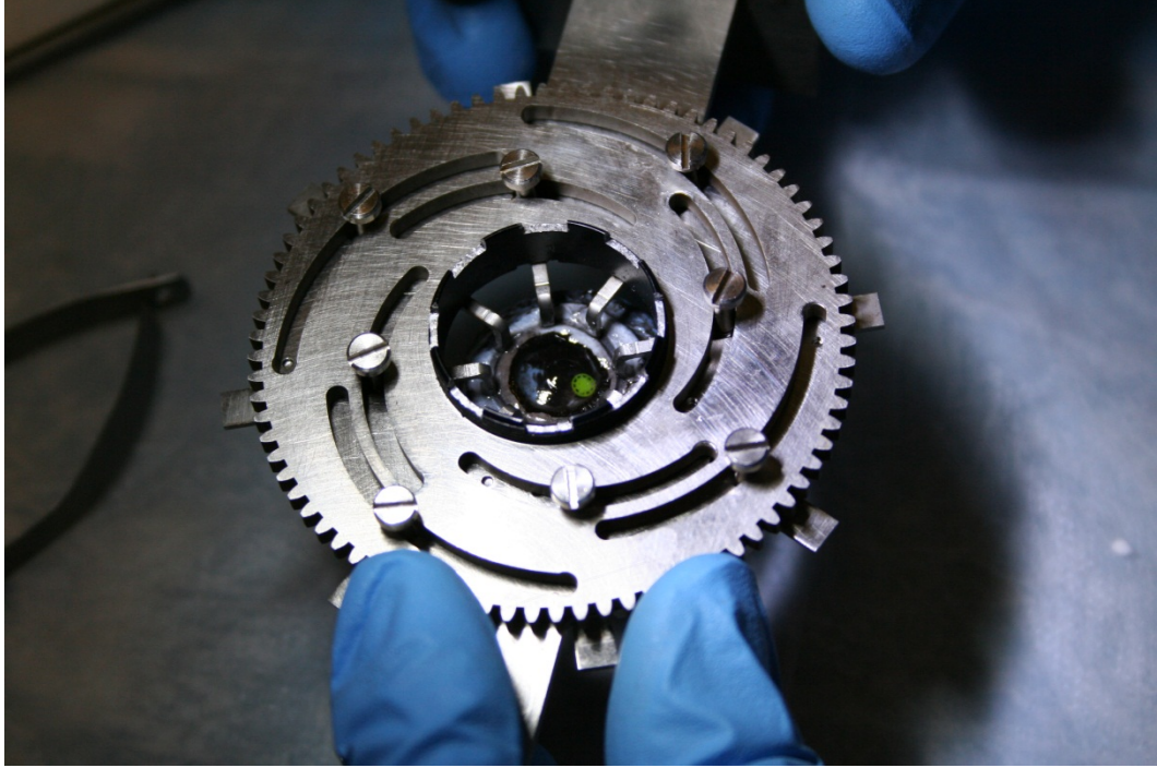
Figure 3-12. Gluing the ciliary muscle to the stretching apparatus. Cyanoacrylate is applied to the jaws of the stretching apparatus before mounting.
