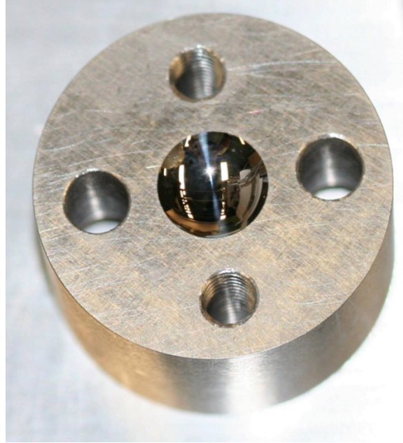
Figure 4-15. One half of the lens mold
