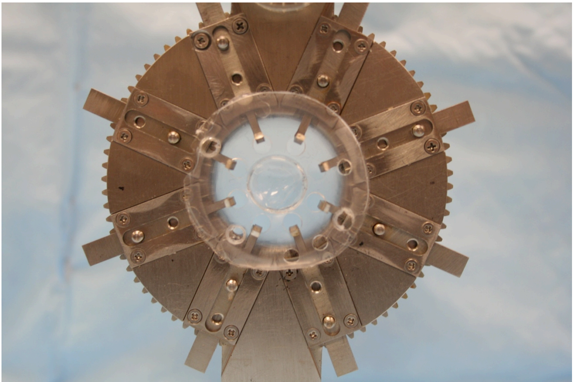
Figure 5-6. Artificial capsule attached to the stretching apparatus with no lens implanted
