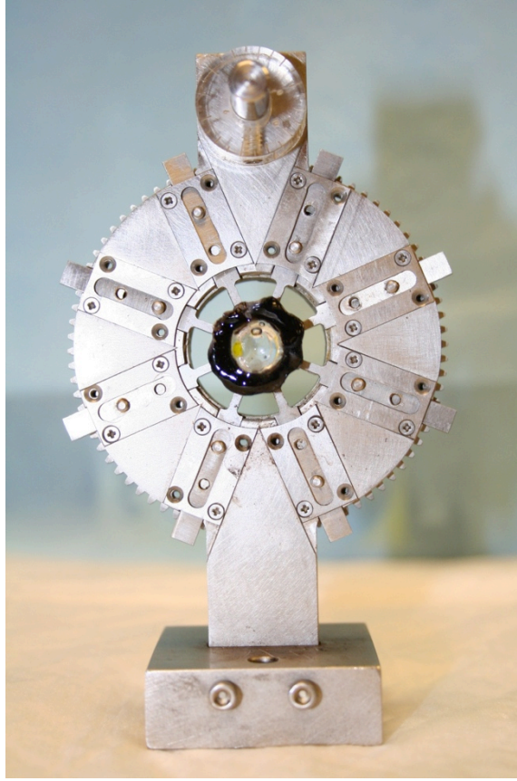
Figure 3-13. Lens mounted and prepared for optical testing
